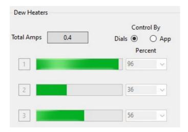
The bottom right quadrant of the application allows the controlling and monitoring of three dew heater outputs.
