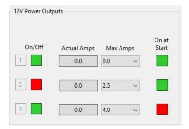
Each 12V output uses a Hall effect current sensor to monitor the output current. This method places almost zero resistance in the current path and so doesn't require large sense resistors. However, it is only accurate to about +/- 0.1A. This means it may show, for example, 0.1A when it should show 0.0A or 0.2A.
