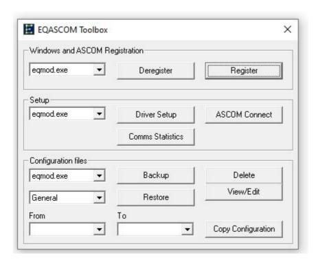
In the Setup box, ensure eqmod.exe is shown and then click on Driver Setup. The EQMod ASCOM setup box will appear.
