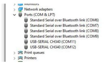
All 4tronix products use the CH340 USB to serial converter chip, so when identifying a COM port, you only need to check the ports that have this name. In the list above, you can see COM11 and COM12 are both showing CH340 as the connection. The correct Port is one of these two.
