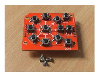
Today you get to fit the final part, a keypad which you can use to control and program your robot. To fit it, place it over the 4 pillars you fitted yesterday and push it down into the black connectors. You will need to have removed the side cables. Screw the keypad into place using the 4 screws provided, then refit the side cables. See next page for programming instructions.
