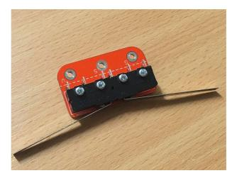
This little sensor assembly is made using 2 microswitches which can be used to detect obstacles in front of Santa's Sleigh. We don't want it crashing into things do we?
