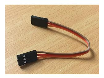
This cable connects the main board to the left side piece. It carries the power and the signal for the multi-coloured LEDs. Connect from the main board (front Right) to the top set of 3 pins on the left side. The Brown wire should be at the front of the robot for both connectors – ie. do not twist the cable. After this cable is connected, the LEDs on the left side will flash different colours with the different directions that the wheel moves.
