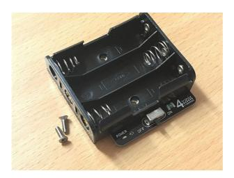
The battery holder comes with two small screws which will be screwed into the top of the hexagonal pillars that you fitted yesterday. But first, you need to plug in wires from the motors into the white sockets in the rear corners of the chassis. They will only fit one way round, so you can't plug them in incorrectly.
