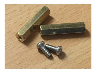
Use the screws to fit the 20mm hexagonal pillars into the 2 holes provided. One, directly between the motors and the other close to the rear edge. Tighten the screwsfirmly.
