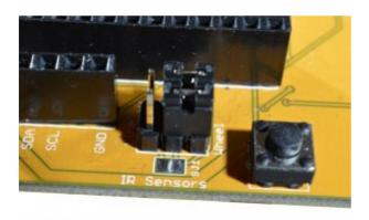
\*\* v1.0 Only Ensure you have cut the 2 tracks as described in step 3. It is really difficult to cut the tracks after the jumper block is fitted.
