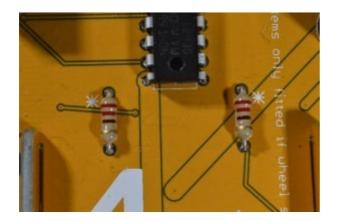
These can be soldered into the middle of the board in positions marked with an asterisk.
