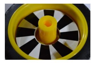
I prefer to use 5 drops of superglue - one on each spoke of the wheel. Then drop the encoder disc into each wheel as shown, with the black/white markings uppermost. Leave to dry while you get on with the soldering.
