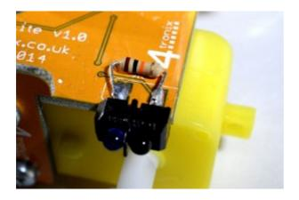
As when building the Pi2Go-Lite kit originally, you should cut the pins on the sensors, next to the flattened part on the legs. Then solder them on.
