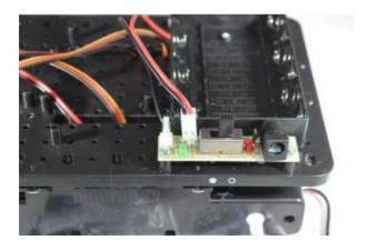
\*\* It is very important to attach this to the correct connector as shown above (labelled "batt"). Please double-check this before connecting batteries
