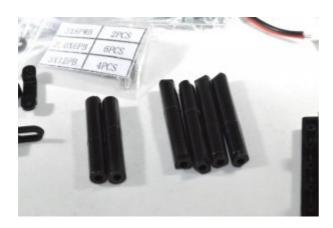
There are six 40mm pillars in the kit. 4 of them have flattened ends and 2 of them are straight. The 4 with flattened ends are to support the upper plate, so select the 2 straight ones for this task.
