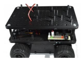
Ensure the flattened ends at the top of each pillar fit into the recesses in the top plate, then use the remaining 4 screws to tighten the plate in position
