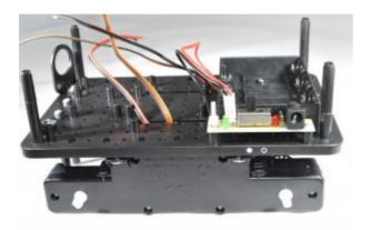
Screw the 4 pillars in tightly from underneath, ensuring that the flattened ends fit snugly into the recess in the plastic plate
