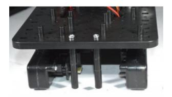
Screw the pillars in place. Note: you can vary the separation of the line following sensors by mounting the pillars in different holes, or to a lesser extent by twisting them once fitted
