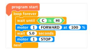
In this example, motor 1 runs forward for 5 seconds every time the button is pressed (C goes HI).
