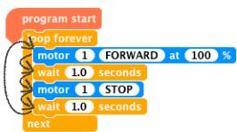
Once the Crumble reaches the last instruction within the loop forever' block, the Crumble will jump back to the top of the loop and repeat the instructions (see the step-by-step example on the next page).
