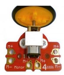
This requires the two terminals on the Crumb to be connected to the Motor1 or Motor2 outputs on the Crumble
