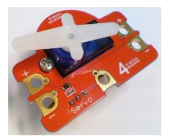
This requires Power and Ground to be connected as well as the centre connection to one of the outputs on the Crumble
