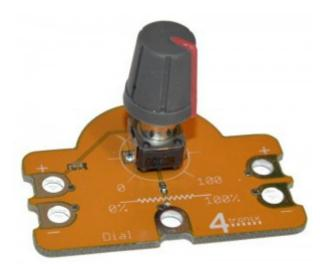
This requires Power and Ground to be connected and the output connected to A, B, C or D. The analog value read will be in the range 0 to 255, though in practice the power is not at 5V so the top end number will be lower
