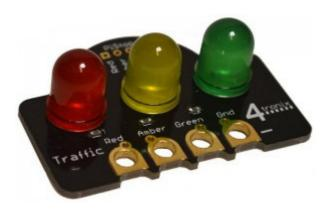
This requires the Ground to be connected and the Red, Amber and Green connections made to your choice of A, B, C or D on the Crumble
