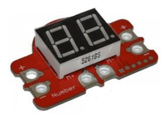
This requires Power and Ground to be connected as well as M+ and M- to be connected to the Motor1 or Motor2 outputs on the Crumble
